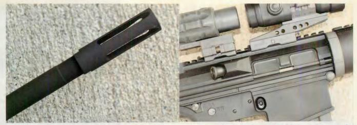
(left) Another feature standard on the LR308 is DPMS' own flash hider screwed on the end of its M4 style barrel. (right) DPMS's LR308 upper receiver features a combination case deflector/forward assist.
